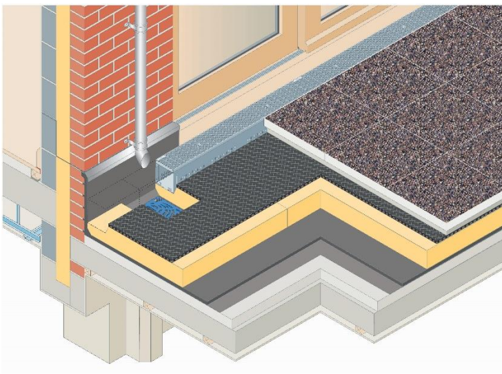
Paved deck on drainage mat
